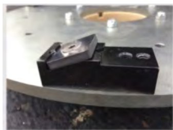
Standard Blade Mount for Wide Cutting Edge
