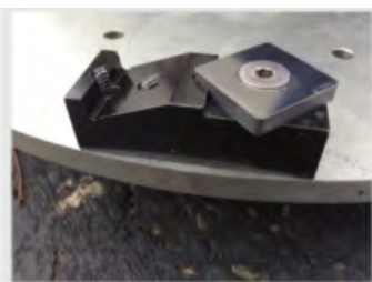
45° Mount for Sharp Cutting Point
